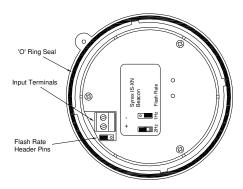
Fig 1 Location of field terminals and controls.
